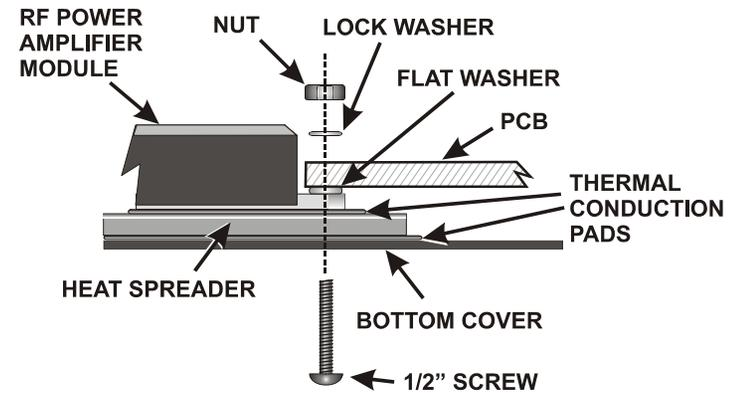
**Figure 42. RF Amplifier Module Mounting Hardware.**
