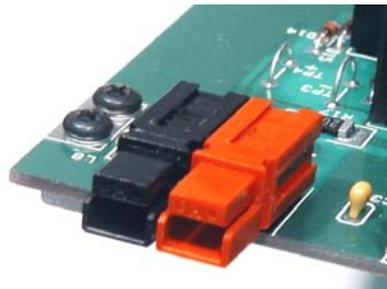
**Figure 28. Orienting J7 on the RF PCB.**
