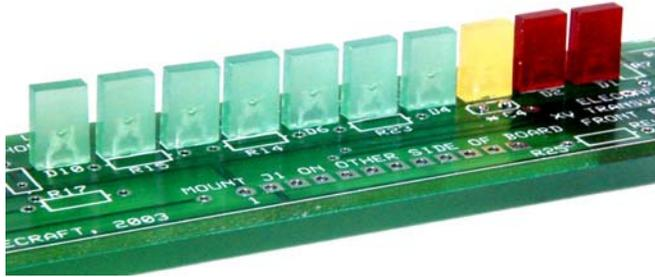
Figure 11. Power LEDs Installed on Front Panel PCB.
