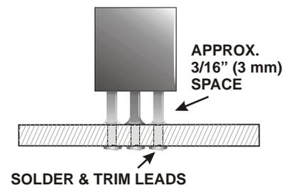
Figure 8. Installing Transistors.
