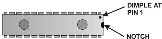
Figure 45. IC Orientation.
