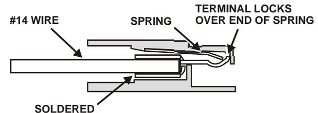
**Figure 26. Inserting Terminal into Anderson Connector Housing.**
