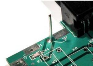
**Figure 29. PCB Antenna Connection.**
