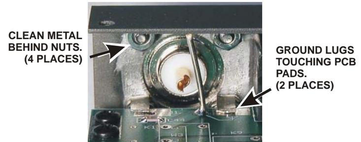
**Figure 32. Mounting Antenna Connector J1.**
