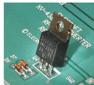
**Figure 22. Installing Transistor Q4.**
