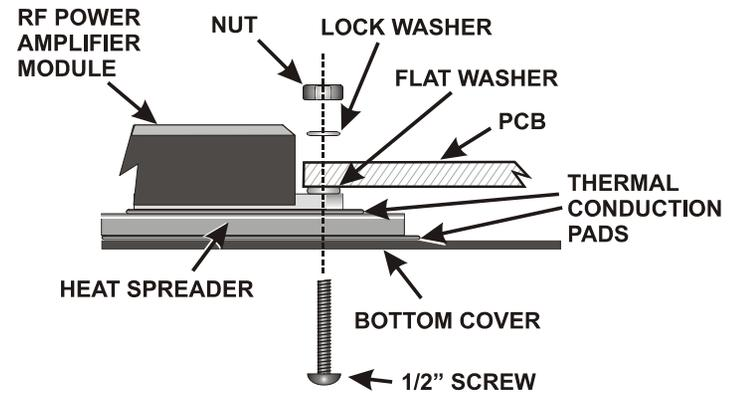
**Figure 42. RF Amplifier Module Mounting Hardware.**
