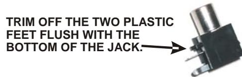
**Figure 24. Preparing the RCA Jacks for Installation.**
