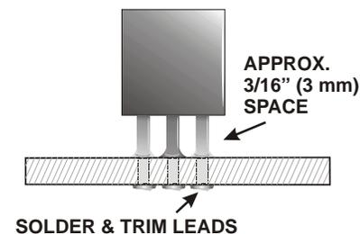
Figure 8. Installing Transistors.
