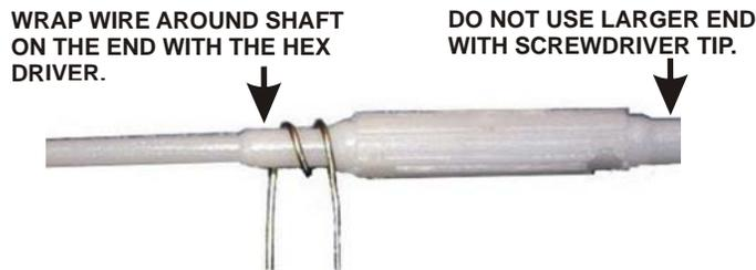
**Figure 34. Winding L10 on the Alignment Tool.**
