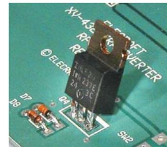
**Figure 22. Installing Transistor Q4.**
