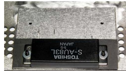
**Figure 39. RF Power Module and Flat Washers in Place on the Heat Spreader.**
