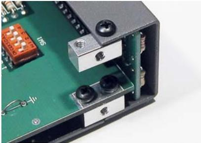
**Figure 46. Attaching 2-D Fasteners to Cabinet End Covers.**
