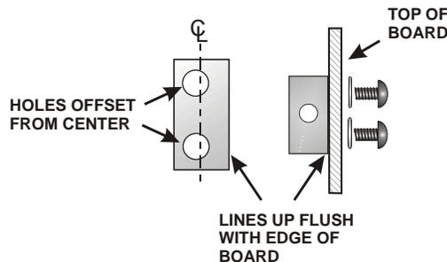
**Figure 31. 2-D Fasteners.**
