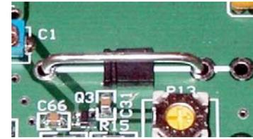
**Figure 21, Inductor L1 Positioned for Soldering.
