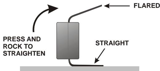
Figure 44. Straightening IC Pins.
