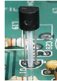
Figure 23. Installing Q1 with Teflon Spacer.
