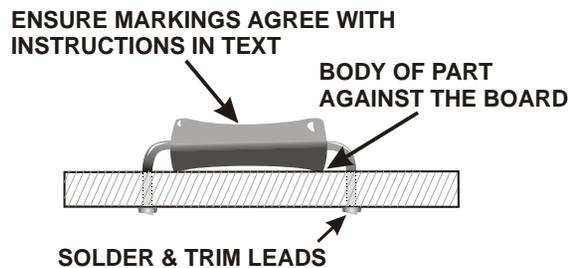
**Figure 12. Installing Resistors.**
