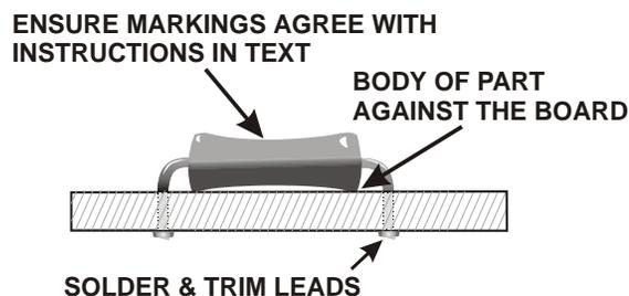
Figure 12. Installing Resistors.
