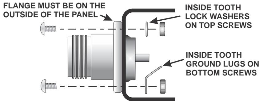
**Figure 30. Mounting the Antenna Connector J1 on the Back Panel.**
