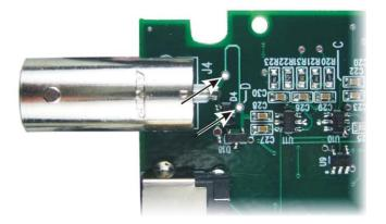
Figure 3. Fusible Trace Solder Pads.
