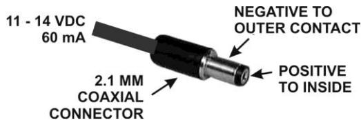
Figure 2. External Power Connector
