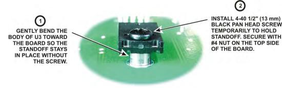
Figure 2. Installing U3 Spacer.
