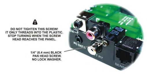
Figure 8. Installing PTT RY Connector Screw.
