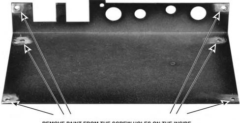
REMOVE PAINT FROM THE SCREW HOLES ON THE INSIDE SURFACE OF THE COVER NEAR THE CORNERS (SIX PLACES)
