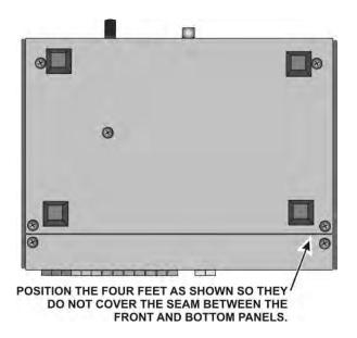
Figure 12. Mounting the Feet on the Bottom Cover.
