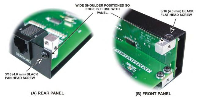
Figure 10. Mounting Front and Rear Panel 2D Fasteners.
