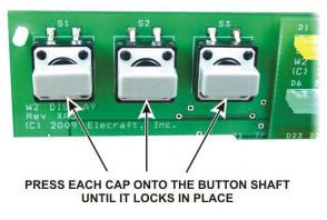
Figure 4. Installing Pushbutton Key Caps.
