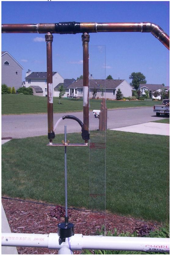
Note the coaxial "jumper" between the two-capacitor pistons...this is the rough-tune coaxial capacitor. The coaxial capacitor can be 4" to 12", depending upon the bands desired (longer lengths for 40 meter operation). Slightly heat the outer insulation and slide the inner braid and insulation in and out of the outer braid to accommodate your desired three bands.
