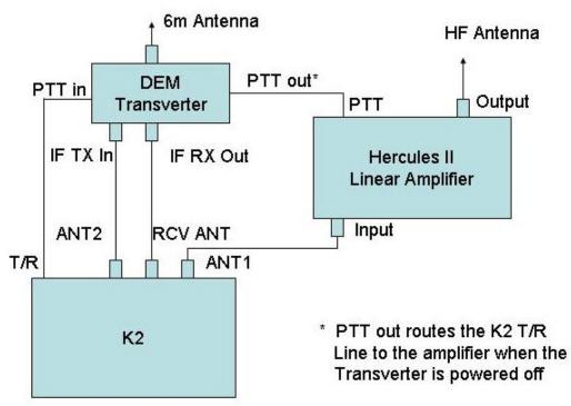
Given that the K2 remembers to select ANT2 and RCV ANT on the transverter band, the only manual operation that would have remained is to disconnect the T/R line from the transverter and switch it to the Hercules II when HF operation with a linear amplifier is desired. This was easily solved by changing the DEM on/off switch to a DPDT, such that whenever the transverter is off, the K2's T/R line is routed out to the linear; when it's on, it controls the transverter.
