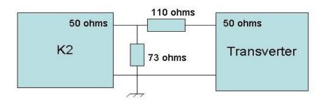
After arriving at the values shown, a trip to Radio Shack found that they were out of many values but had plenty of 220 ohm, 1 watt resistors. I build the attenuator inside the DEM transverter (there is plenty of room) using 3 220 ohm resistors in parallel to ground and 2 220 ohm resistors in parallel between the K2 and the transverter TX/IF input. Close enough!
