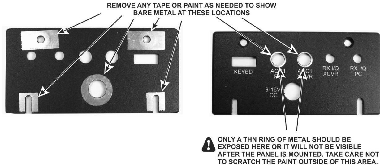
Figure 34. Preparing the Left Side Panel for Mounting.
