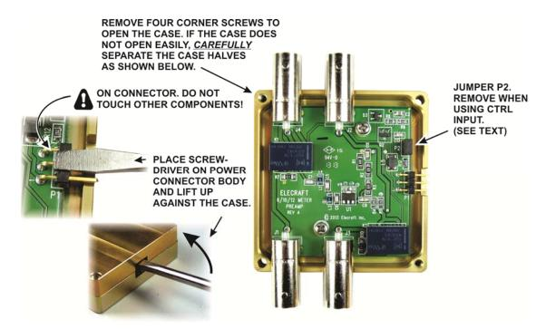
Figure 3. Jumper P2 Location.
