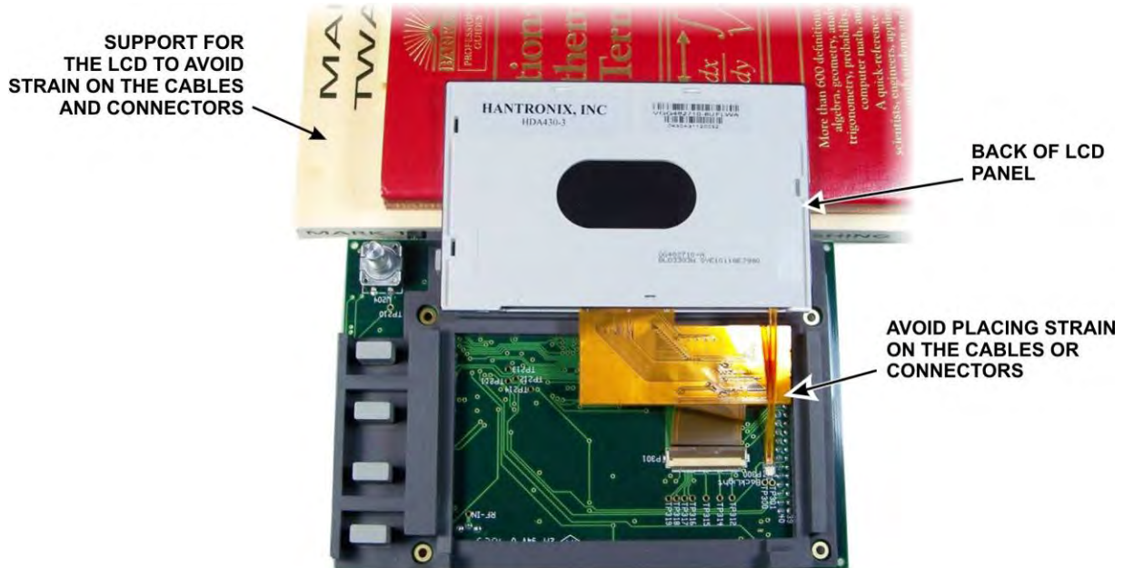
Figure 25. Removing LCD Panel from Rubber Key Matrix.
