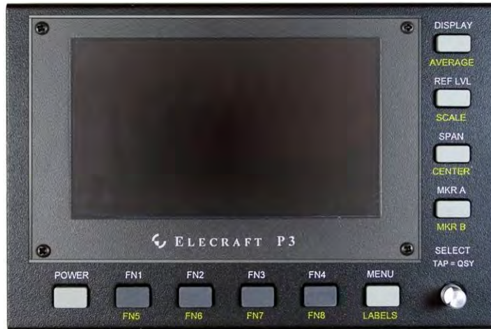
Figure 5. Bezel Mounted on Front Panel.
