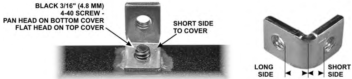
Figure 10. Installing Angle Brackets on the Covers.
