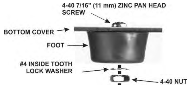
Figure 8. Installing Rear Feet.
