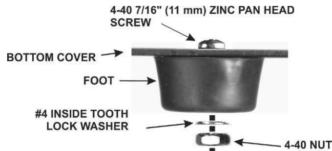
Figure 8. Installing Rear Feet.
