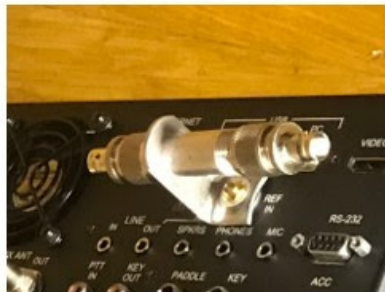
Fig. 2: Whip swivel mount on rear panel
