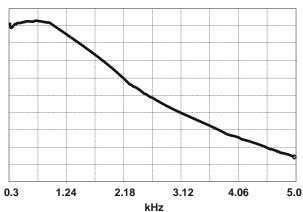
BANDPASS FILTER POSITION 1 LOW PASS FILTER SET TO MAXIMUM BANDWIDTH
