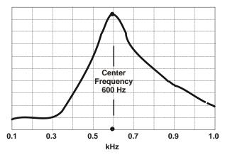
BANDPASS FILTER POSITION 2 LOW PASS FILTER SET TO MINIMUM BANDWIDTH
