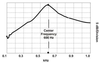
BANDPASS FILTER POSITION 2 LOW PASS FILTER SET TO MAXIMUM BANDWIDTH
