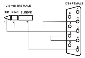
Figure 10. Serial Interface Cable Schematic.
