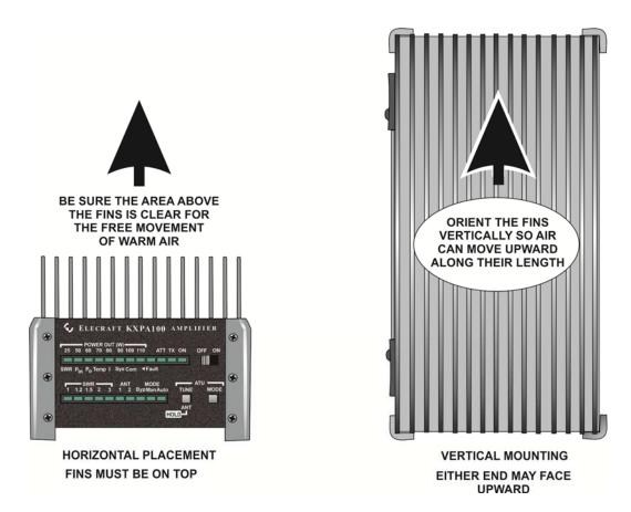
Figure 1. Orienting the Amplifier for Proper Cooling.
