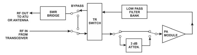
Figure 1 is a simplified block diagram of the amplifier.
