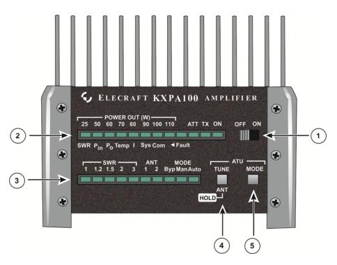
Figure 5. Front Panel Controls and Indicators
