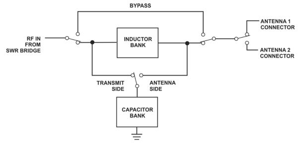
Figure 9. KXAT100 Antenna Tuning Unit Simplified Block Diagram.
