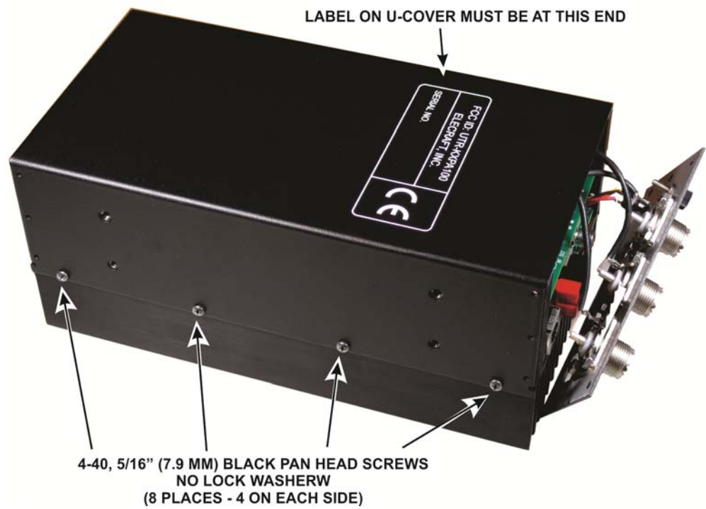
Figure 17. Mounting the U-Cover.
