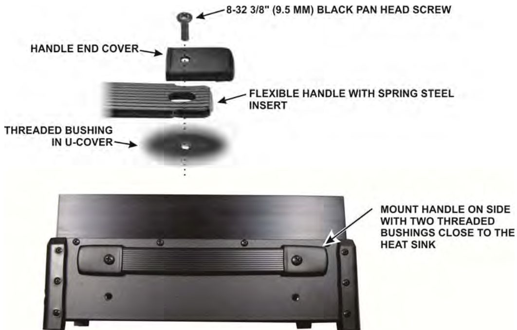
Figure 23. Mounting the Side Handle.
