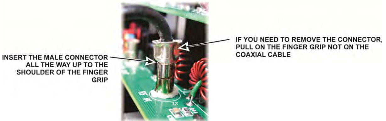
Figure 14. Mating TMP Connectors.
