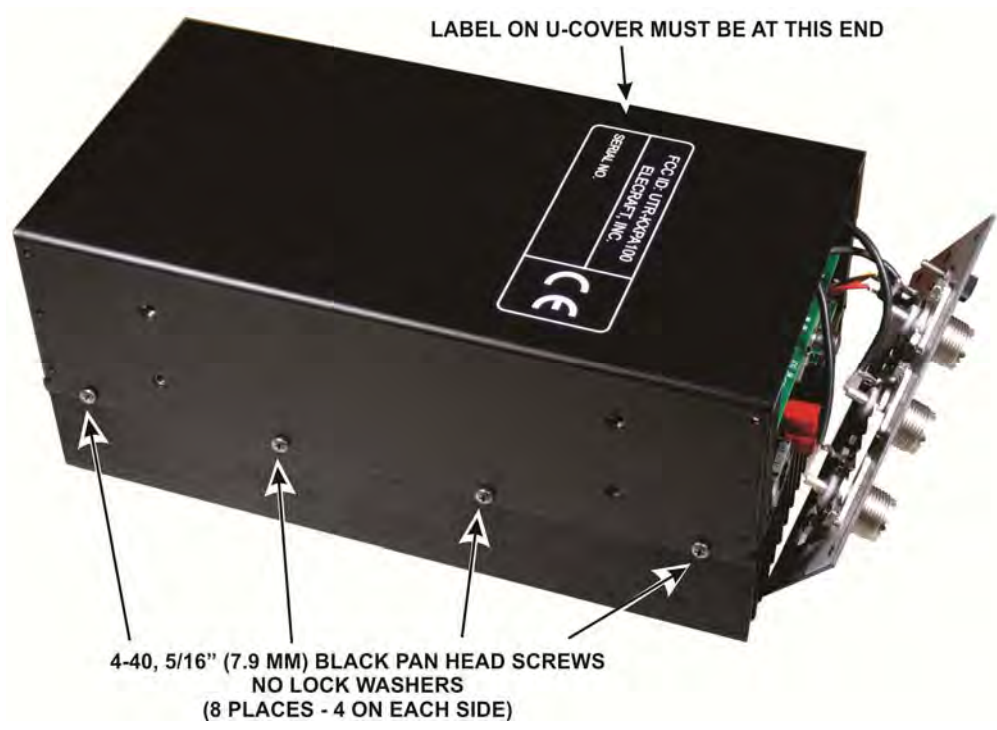
Figure 19. Mounting the U-Cover.
