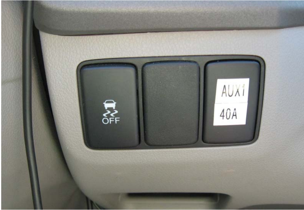
Figure 4. 40A branch circuit power switch on the Civic's instrument panel. There were two "dummies" in this panel, so I removed the rightmost one and filled its slot with a Honda standard switch replacement. The KX3 and mount aren't seen, but they are located directly above this panel. The microphone cable is shown hanging at the left.
