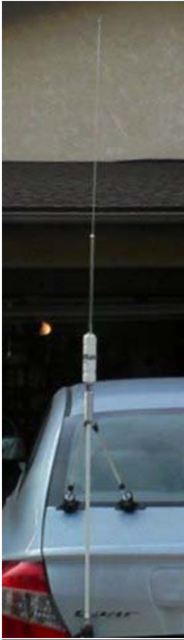
Figure 8. Trunk lip-mounted Hustler short mast with a 40m resonator attached.
