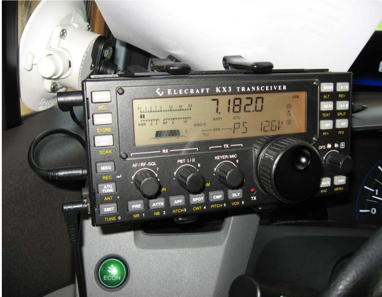
Figure 1. Seasucker 6018 vacuum mount with a KX3 in a Honda Civic. The piece of paper to the KX3's rear was used to block sunlight for purposes of shooting the photograph.
