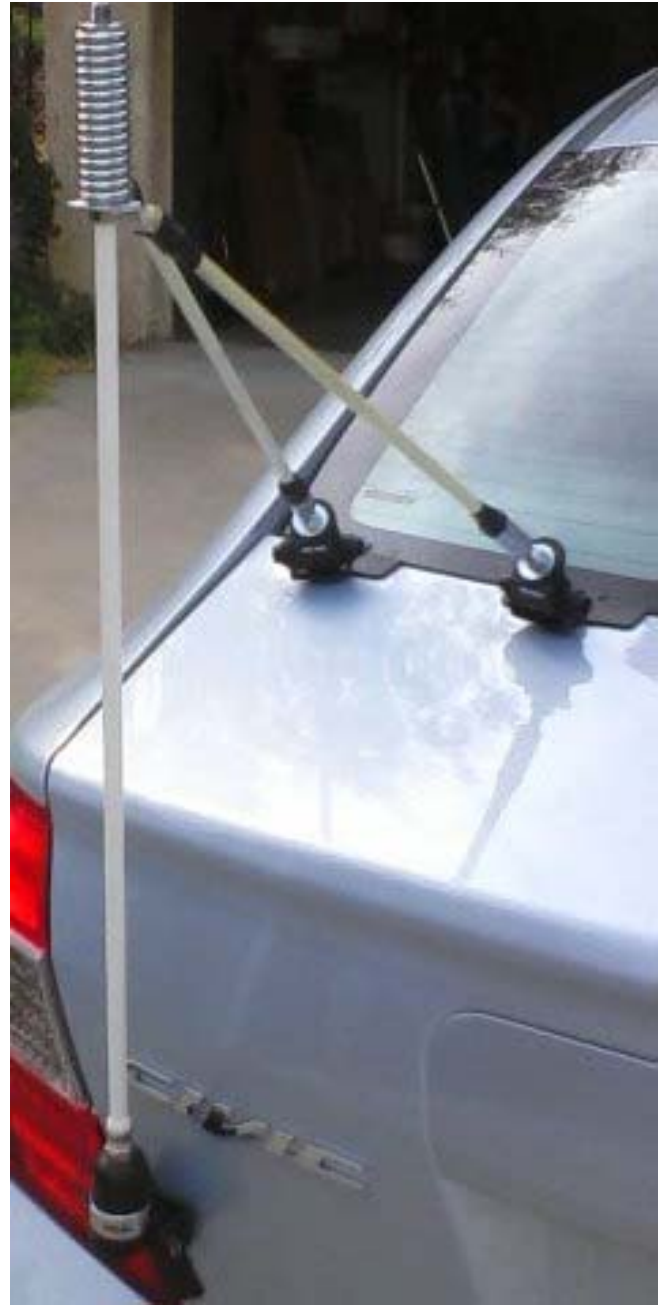
Figure 9. Detail shot of the tripod mount and the Hustler short mast.
