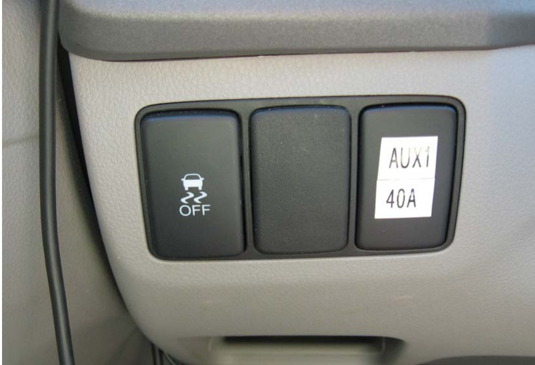
Figure 4. 40A branch circuit power switch on the Civic's instrument panel. There were two "dummies" in this panel, so I removed the rightmost one and filled its slot with a Honda standard switch replacement. The KX3 and mount aren't seen, but they are located directly above this panel. The microphone cable is shown hanging at the left.
