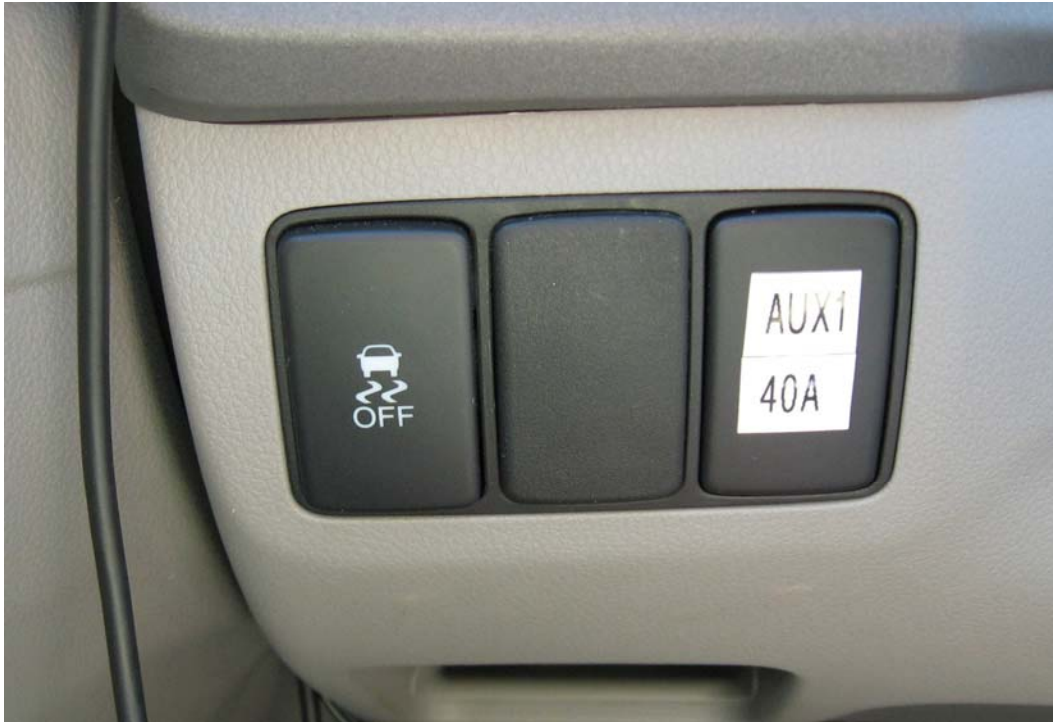
Figure 4. 40A branch circuit control switch on the Civic's instrument panel. There were two "dummies" in this panel, so I removed the rightmost one and filled its slot with a Honda standard switch replacement. The KX3 and mount aren't seen, but they are located directly above this panel. The microphone cable is shown hanging at the left.
