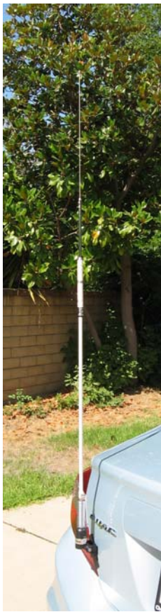
Figure 8. Trunk lip-mounted Hustler short mast with a 20m resonator attached.
