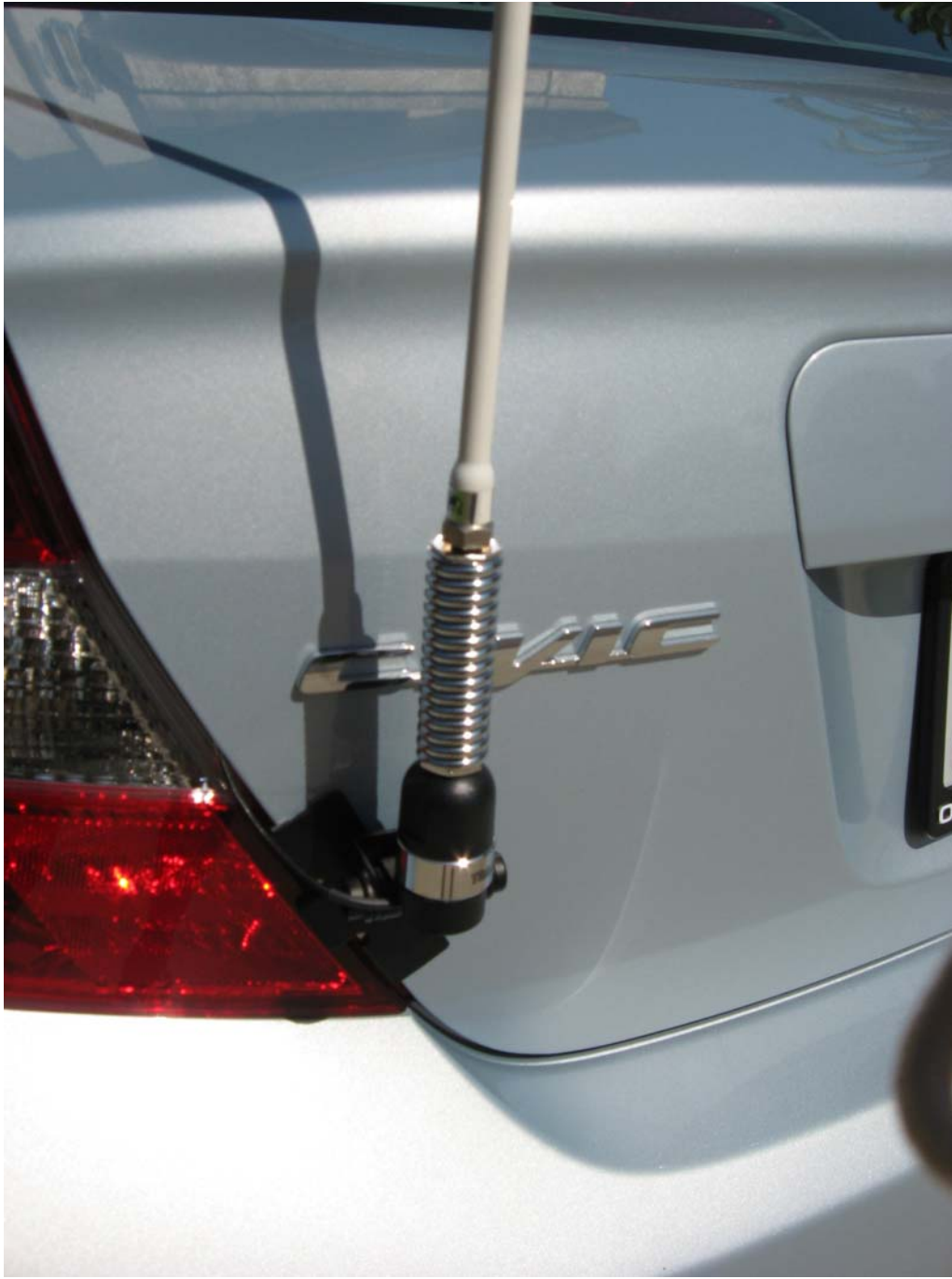
Figure 9. Detail shot of the trunk lip mount and lower section of the Hustler short mast.
