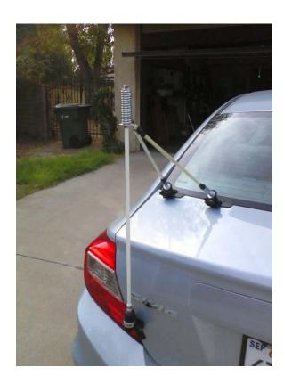
Figure 10. Detail shot of the tripod mount and the Hustler short mast.
