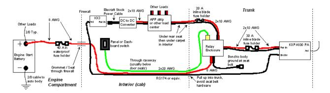
Figure 3. Wiring Diagram: Example of KX3 and KXPA100 power and antenna cabling.
