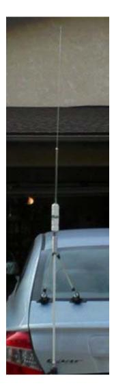
Figure 9. Trunk lip-mounted Hustler short mast with a 40m resonator attached.
