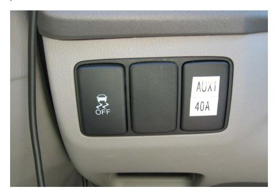
Figure 5. 40A branch circuit switch on the Civic's instrument panel. There were two "dummies" in this panel, so I removed the rightmost one and filled its slot with a Honda standard panel switch replacement. The KX3 and mount aren't seen, but they are located directly above this panel. The microphone cable is shown hanging at the left.
