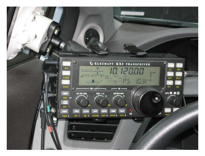
Figure 2. Seasucker 6018 vacuum mount with a KX3 in a Honda Civic. Note the use of the Elecraft KX3-PCKT cable set on the left. The right angle arrangement keeps cable layout tidy and out of the way. Below the audio cables (left side), a retaining clip is used to keep the bundle together.
