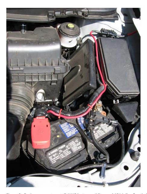
Figure 8. Engine compartment, 8 AWG battery cabling, and 40A inline fuse in fuse holder (upper right). The Motorola fuse holder is waterproof. Unseen in this photo, there is a short length of 5/16" fuel hose slipped over the cable jacket to the right of the fuse holder, to protect it as it traverses several sharp metal edges (weld points).
