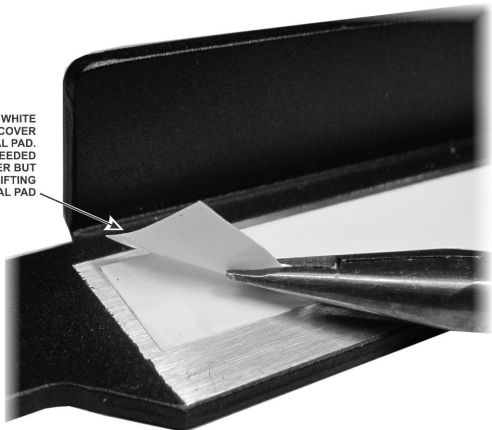
Figure 37. Removing the White Plastic Protective Cover from the Thermal Pad.
