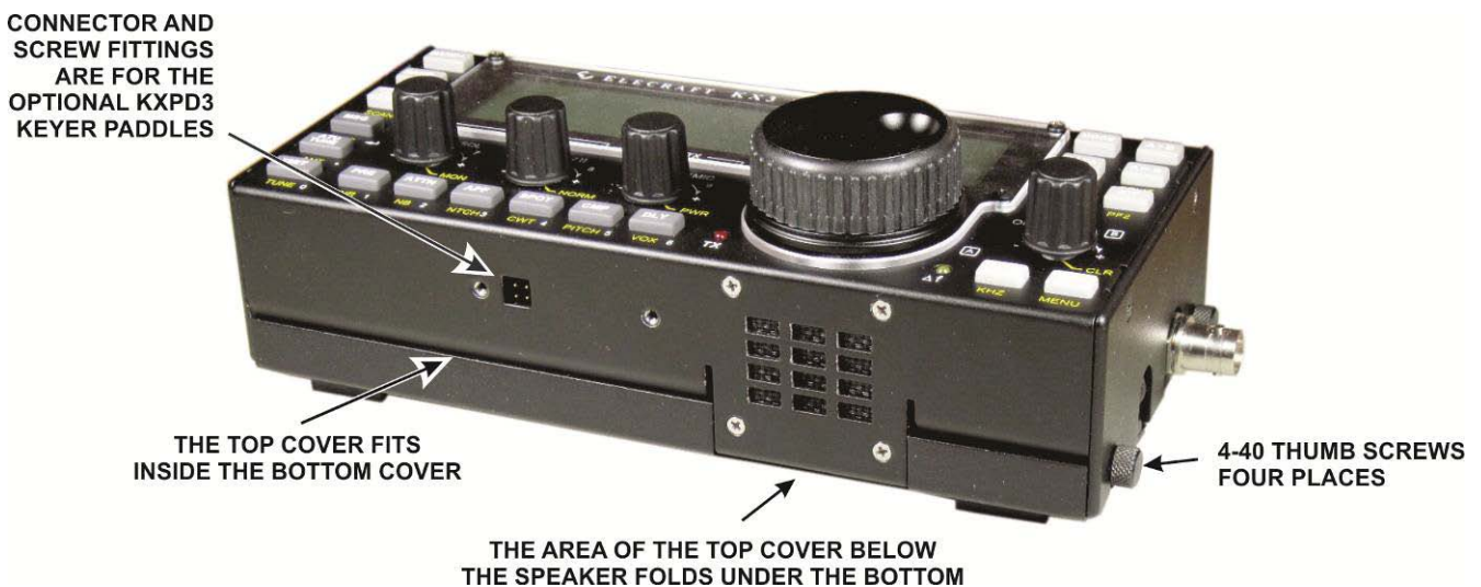
Figure 54. Test Fitting the Top and Bottom Covers Together.
