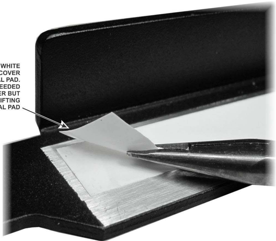
Figure 37. Removing the Clear Plastic Protective Cover from the Heat Sink.
