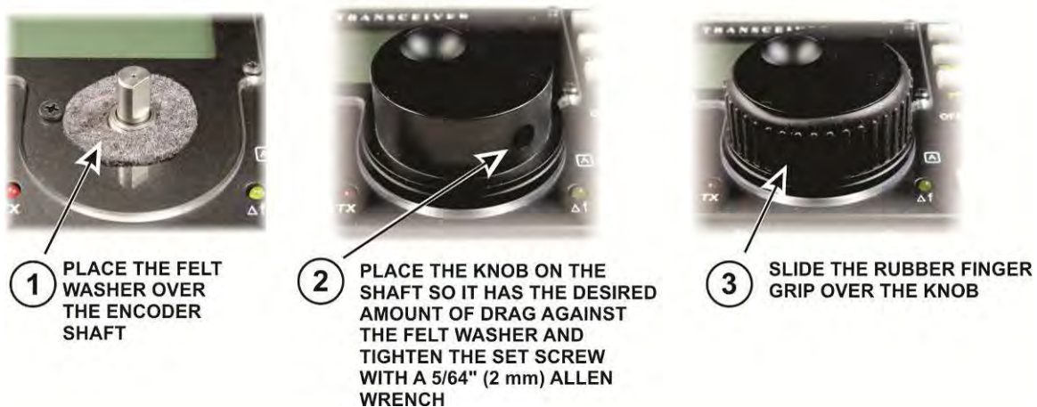
Figure 20. Mounting the VFO Knob.
