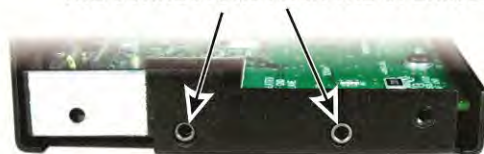
Figure 43. Installing RF Board in the Bottom Cover.
