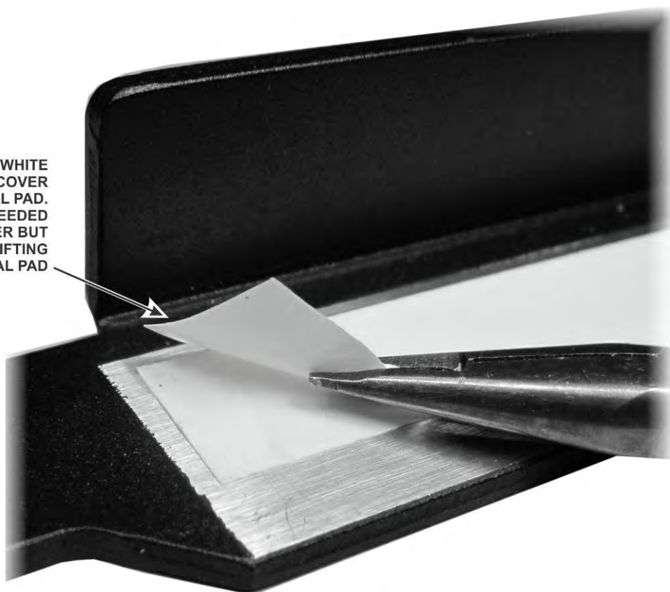
Figure 37. Removing the Clear Plastic Protective Cover from the Heat Sink.
