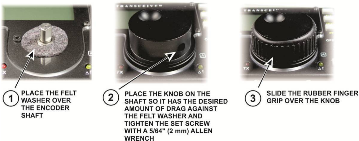
Figure 20. Mounting the VFO Knob.
