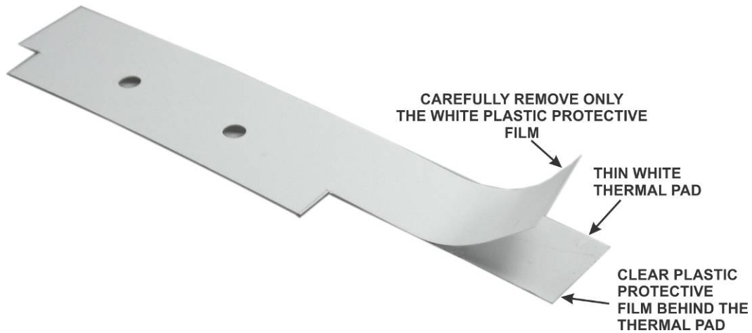
Figure 35. Preparing the Thermal Pad.
