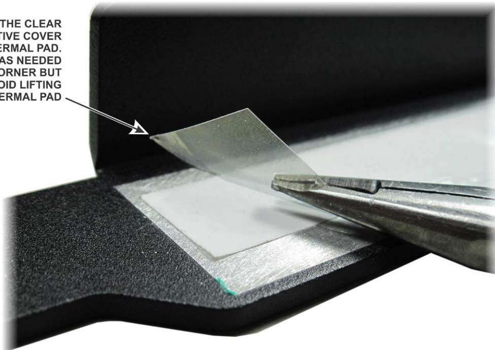
Figure 37. Removing the Clear Plastic Protective Cover from the Heat Sink.
