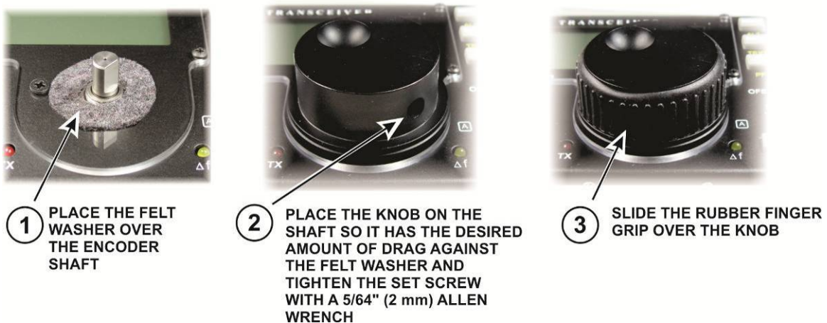
Figure 20. Mounting the VFO Knob.
