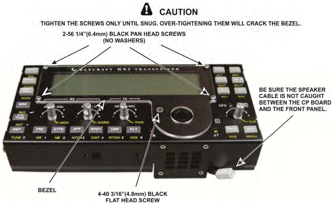
Figure 14. Placing the CP Board in the Front Panel.
