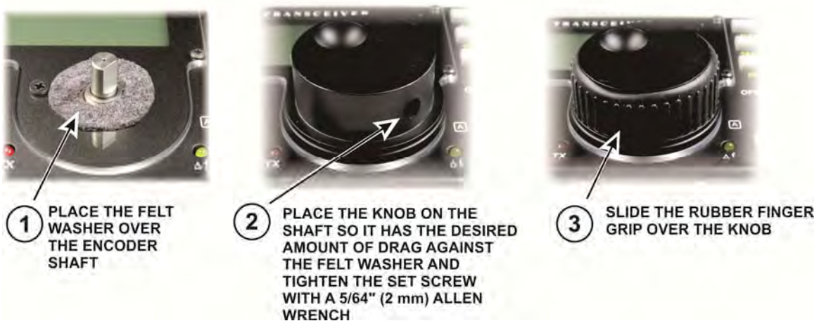
Figure 20. Mounting the VFO Knob.
