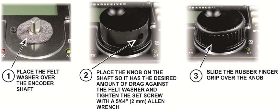
Figure 20. Mounting the VFO Knob.
