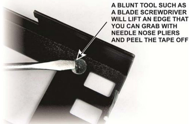
Figure 5. Removing Masking Tape.
