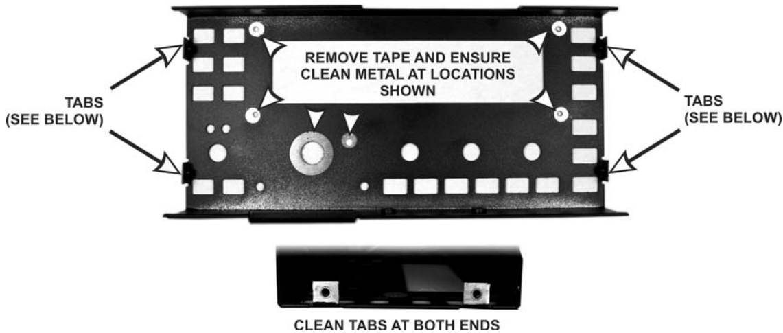
Figure 4. Front Panel Clean Contact Areas.
