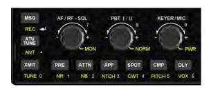
First, tap **FREQ ENT**. Then enter up to three MHz digits, optionally followed by a decimal point (ATU TUNE switch) and up to three kHz digits. Next tap (MSG switch) to accept, or any other switch to cancel. Examples:
