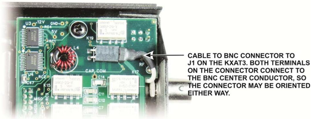
Figure 7. Connecting Antenna Plug to KXAT3 Board.
