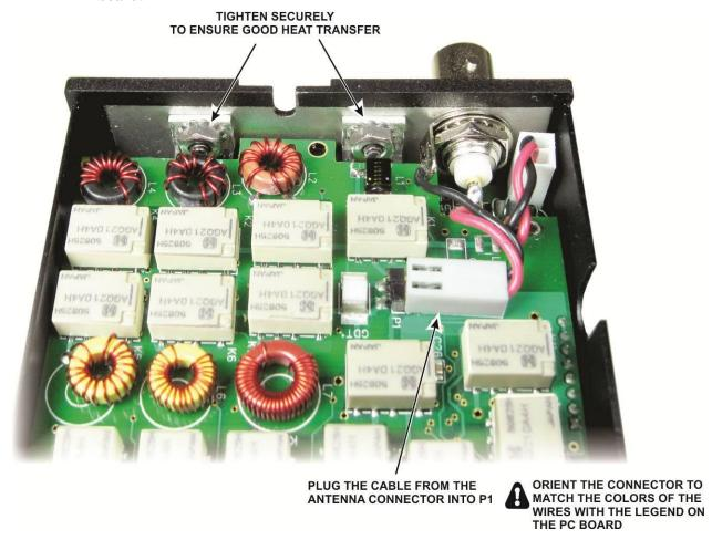
Figure 5. Finishing KXAT2 Installation
