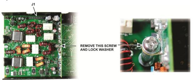
Figure 3. Removing Retaining Screw and Lock Washer.
