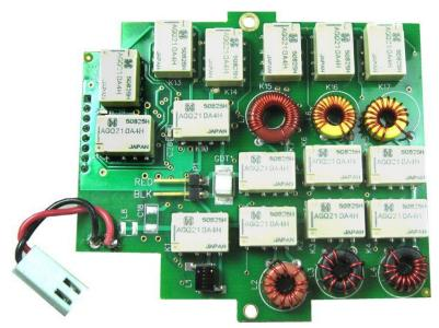
KXAT2 Antenna Tuner Option Circuit Board
