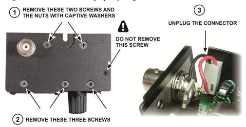
Figure 2. Removing the KX2 End Plate.
