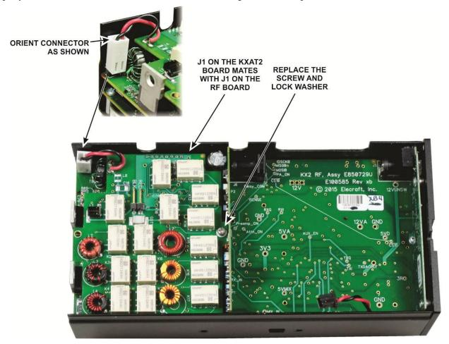
Figure 4. Mounting the KXAT2 Board.
