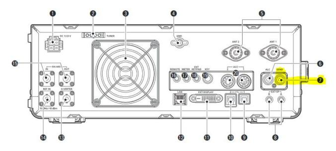
The SEND signal will be used to key the KPA500 and is the same signal routed through the KAT500 to prevent hot switching. Please see the wiring diagram below to see how the connections will be made.
