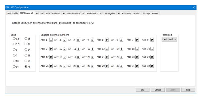
Figure 2. Enable antennas 11 – 16. Disable physical (SO-239) jack ANT 2.
