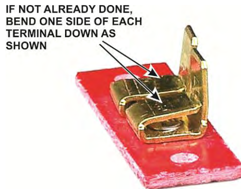
Figure 17. Preparing the Terminal Strip Board.
