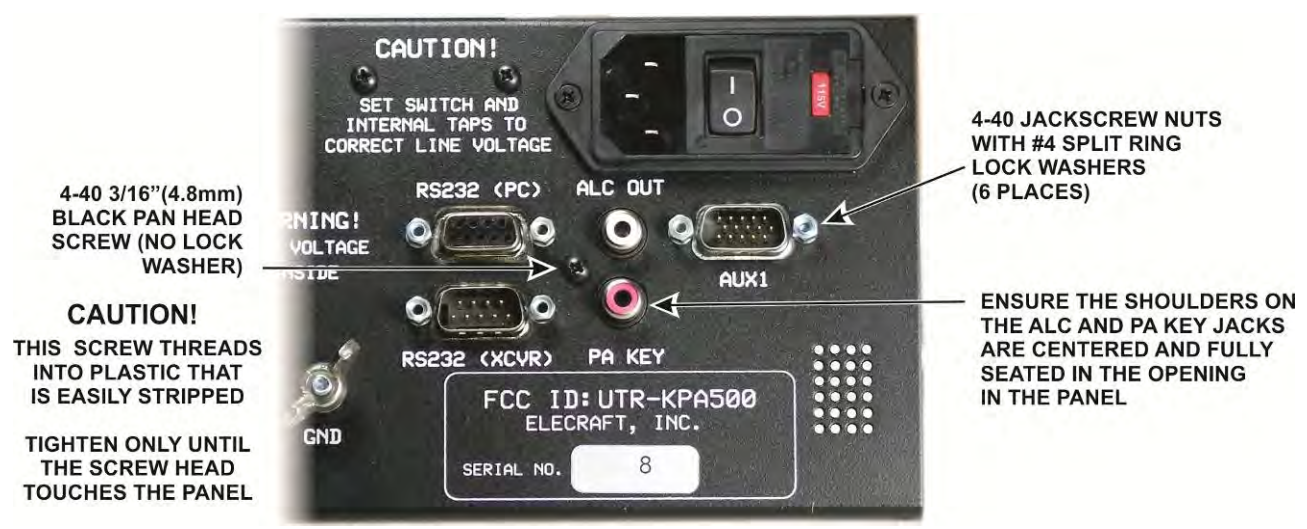
Figure 25. Installing the I/O Module in the Rear Panel.
