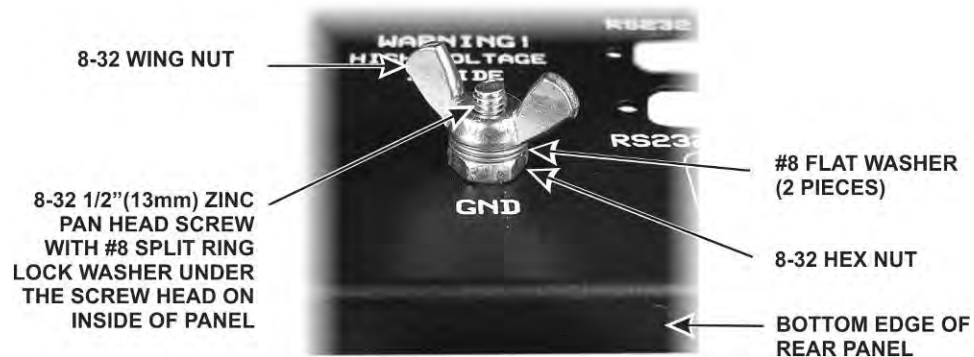
Figure 21. Installing the Rear Panel Ground Lug.
