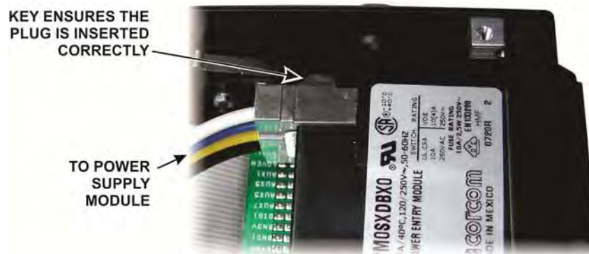
Figure 41. Connecting the 4-Wire Cable to the Power Entry Module.
