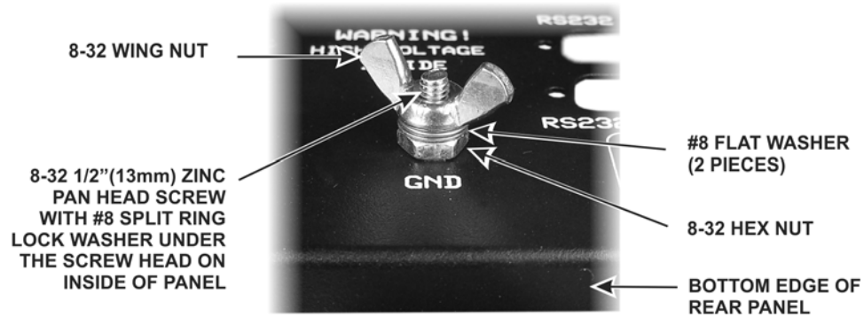
Figure 21. Installing the Rear Panel Ground Lug.
