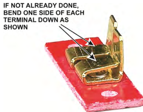
Figure 17. Preparing the Terminal Strip Board.
