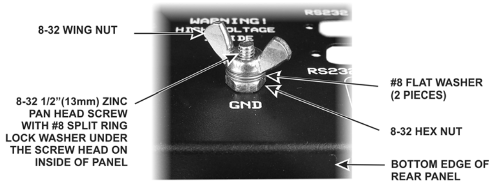
Figure 21. Installing the Rear Panel Ground Lug.
