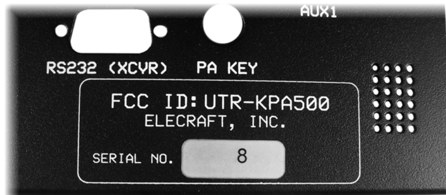
Figure 16. Mounting the Serial Number.
