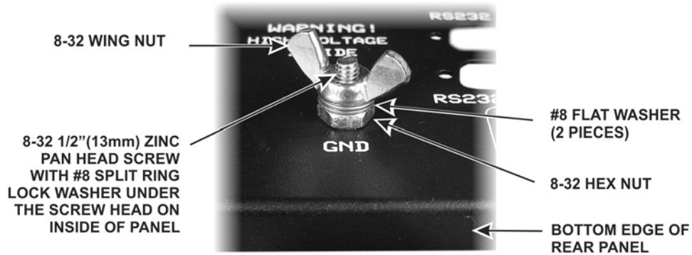
Figure 21. Installing the Rear Panel Ground Lug.
