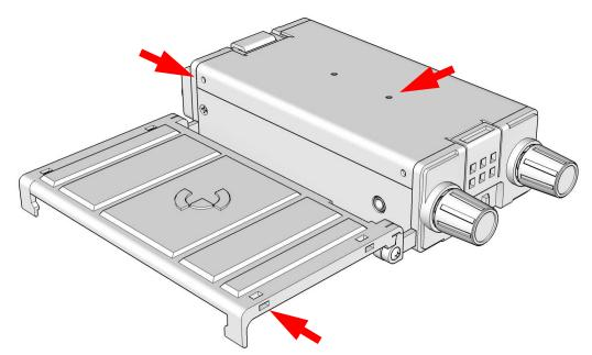
**BACK COVER, MIDDLE:** There are two #2 flat head screw holes in the middle of the back cover. The screw heads must go on the inside, and must be flat head to clear the Li-ion battery pack.
