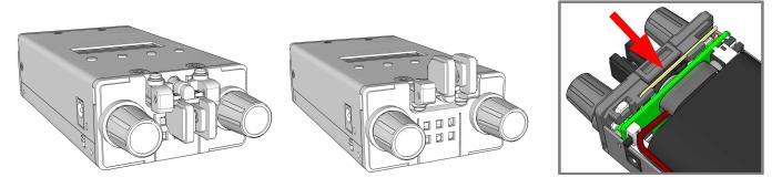
Contact spacing of the KHPD1 paddle can be adjusted using the hex wrench stored inside the enclosure (see arrow in the illustration above-right). Each paddle has a set screw in its housing. A fairly wide spacing is recommended for operation in high-vibration or less-stable operating positions.
