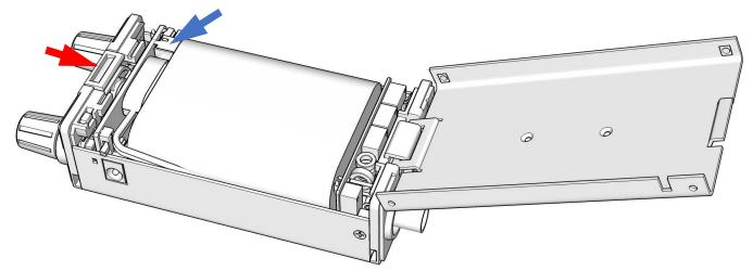
The aluminum back cover has a tab that forms a hinge with the plastic top panel. Once the back cover has been rotated to a perpendicular position, slide its metal tab backward about 1/8" (3 mm) before continuing rotation. This will make it easier to close the back cover.
