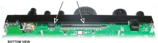
Figure 14. Mounting the Front Panel Assembly- Mating P30 and P35.
