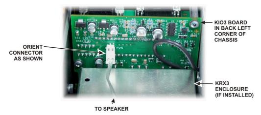
Figure 16. Connecting Speaker Cable.
