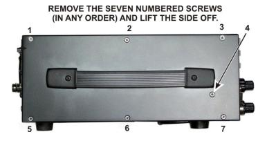
Figure 2. Removing the Left Side Panel.
