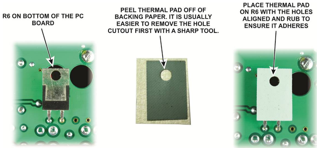
Figure 15. Placing Thermal Pad on R6.
