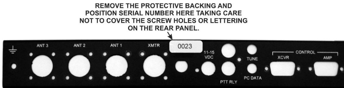
Figure 19. Attaching Serial Number to Rear Panel.
