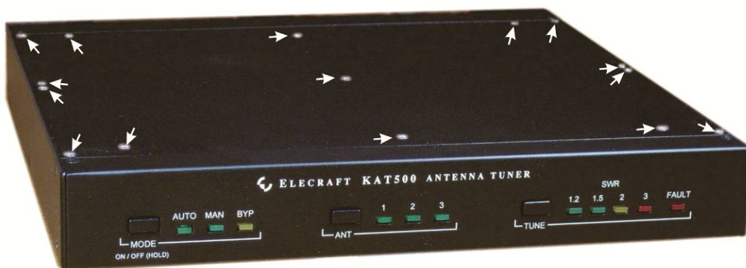
Figure 36. Installing the Top Cover.
