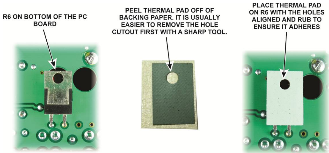
Figure 15. Placing Thermal Pad on R6.
