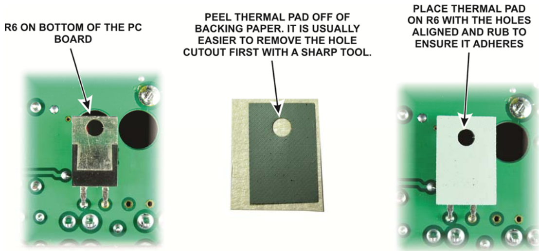
Figure 15. Placing Thermal Pad on R6.
