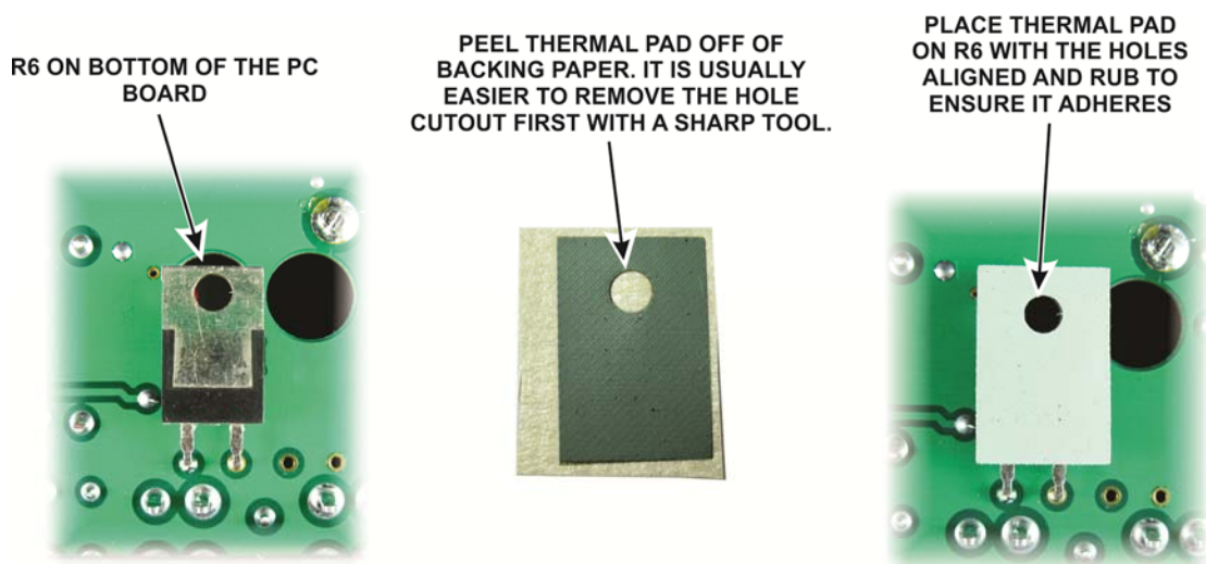
Figure 13. Placing Thermal Pad on R6.
