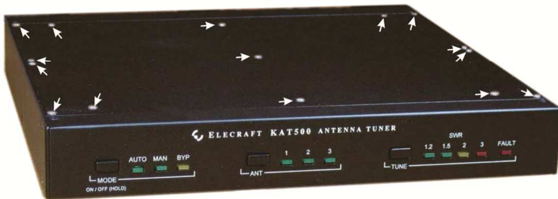
Figure 34. Installing the Top Cover.
