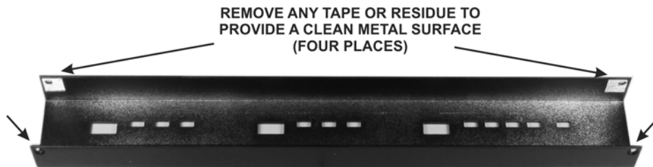
Figure 29. Preparing the Front Panel for Installation.
