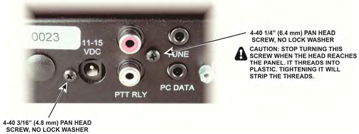
Figure 23. Installing Rear Panel Pan Head Screws.
