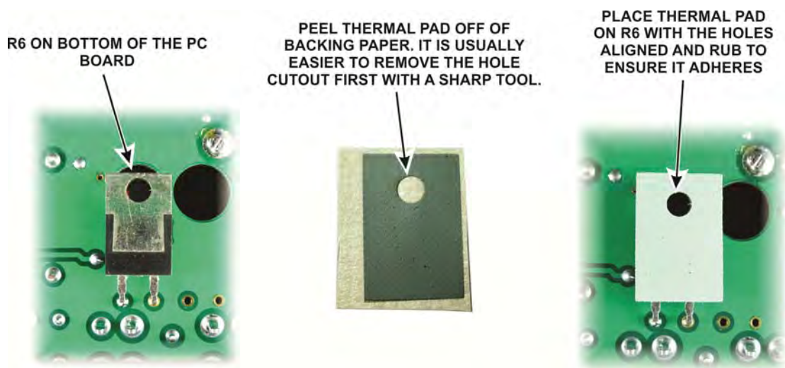
Figure 12. Placing Thermal Pad on R6.
