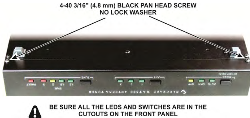
Figure 29. Mounting the Front Panel.
