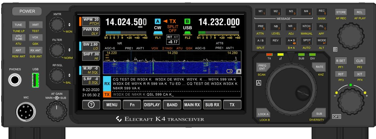
The example below shows the flexibility of the K4's symmetrical user interface, with both dual panadapters and dual text decode selected. The operator can send/receive text in the same or different modes on both VFOs.
