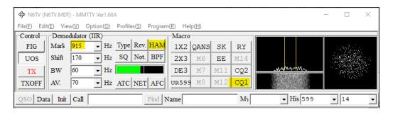
24. Set the K4 MODE to FSK. Tap MAIN RX > LINE OUT and rotate the VFO A knob to adjust the LEFT channel LINE OUT level so that band noise appears at the bottom of the MMTTY spectrum display as shown above.
