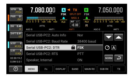
22. When using MMTTY or other external decoders, set FSK Dual-Tone RX Filter to OFF, and FSK Polarity to NORM. Tap the K4 S-Meter to display the K4 Mini-Pan which has vertical lines to to assist with centering RTTY signals in the K4 passband
