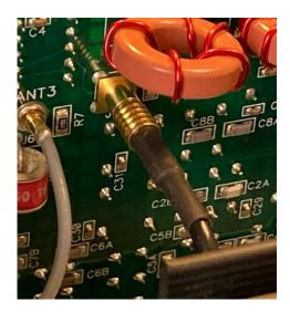
12. The right-angle MCX end is inserted into a connector on the main board below, into a jack labeled "Non-TX ANT" located between the two fans and the KPA4 (black heatsnk).
