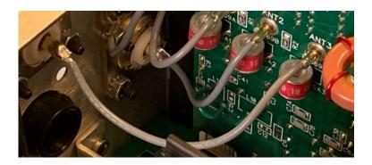
11. Locate the black cable with the gold connectors on each end. One end has a straight MCX connector, the other has a right-angle MCX connector. The straight end goes into the gold connector on the KAT4 labeled "J4", next to "ANT3".
