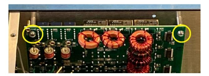
8. Now connect ANT1's center wire to the "ANT1" socket on the KAT4, and the ground wire to the "GND" socket.
