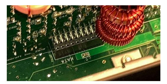
7. Secure the KAT4 board with the two zinc screws in the holes shown below circled in yellow. If the screws don't go in easily, you should check the alignment of the board in the connector. It may be offset in one direction.
