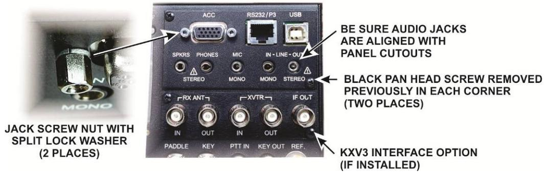
Figure 8. Mounting the new KIO3B Rear Panel Cover.
