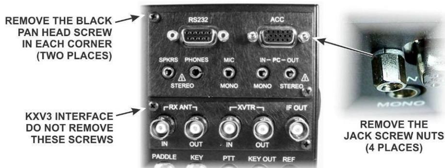
Figure 3. Removing the KIO3 Rear Panel Cover.
