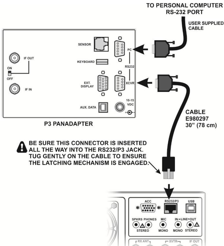
Figure 13. P3 Cabling for RS232 Computer Interface.
