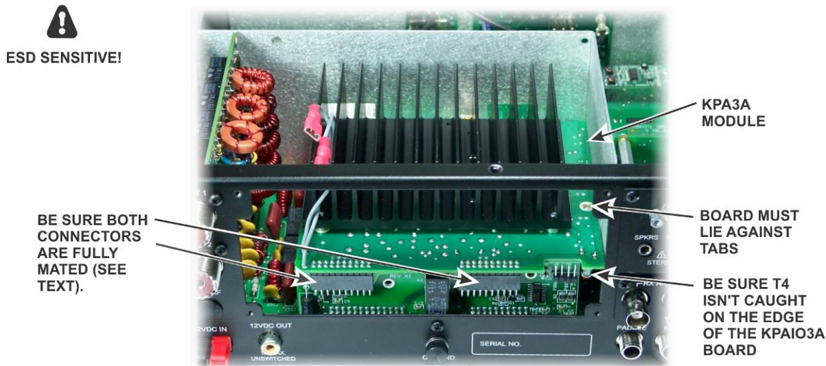
Figure 15. Mounting the KPA3A Module.
