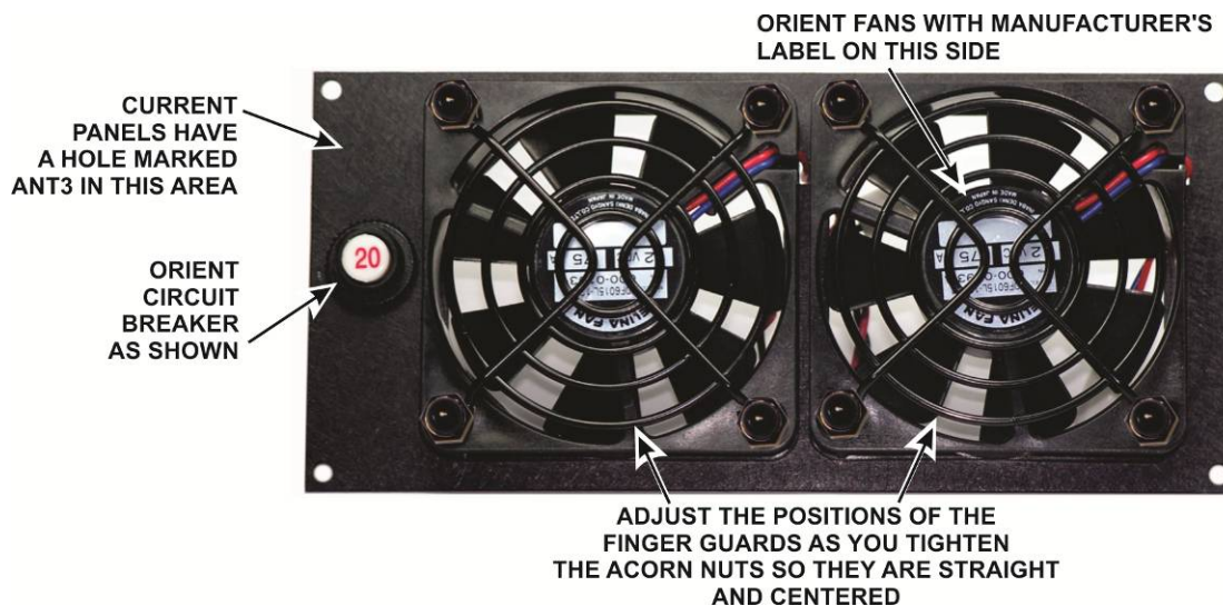
Figure 13, Completed Fan Panel from Rear.
