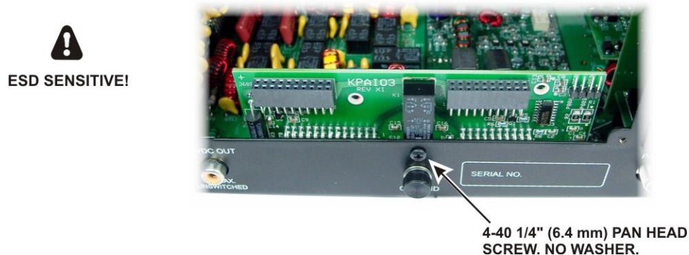
Figure 11. Installing the KPAIO3A Module.
