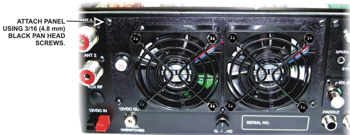
Figure 17. Fan Panel Installed.
