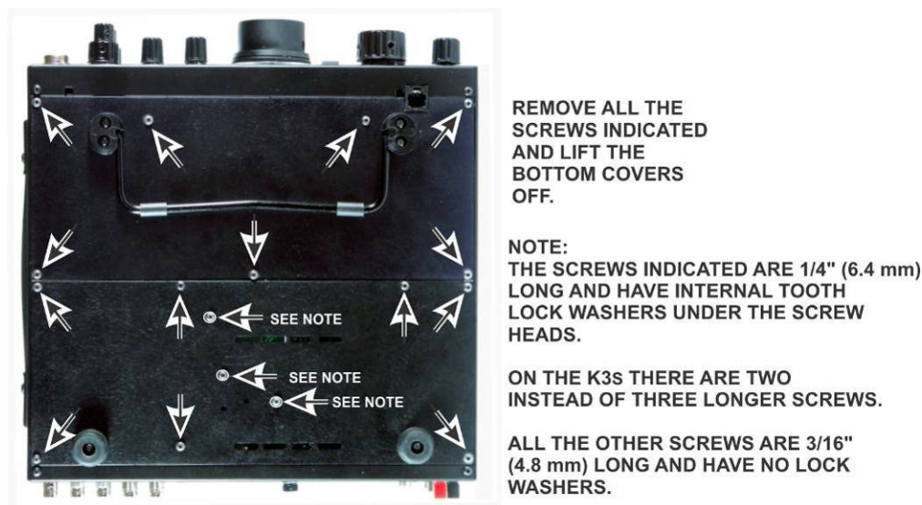
Figure 11. Removing K3s/ K3 Bottom Cover.
