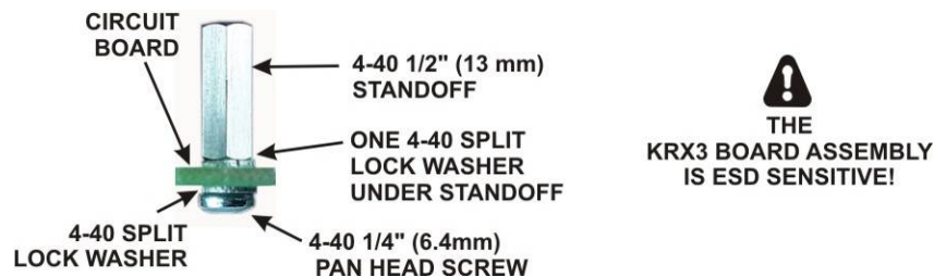
Figure 7. Installing the Standoffs.
